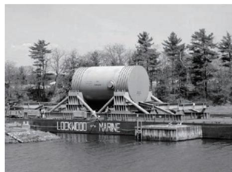
Fig. 2 Maine Yankee RPV ready for transport to Barnwell by barge
