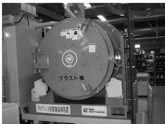
Fig. 4 Dry blasting decontamination apparatus
