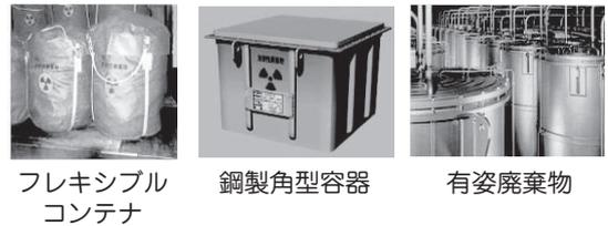
Fig. 5 Examples of waste packages for trench-type disposal facility
